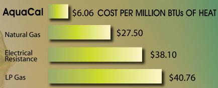
\*Chart based on \$3.00 per gallon LP Gas, \$2.20 per therm. of Natural Gas, 13¢ per kilowatt and a heat pump with C.O.P. of 6.3
