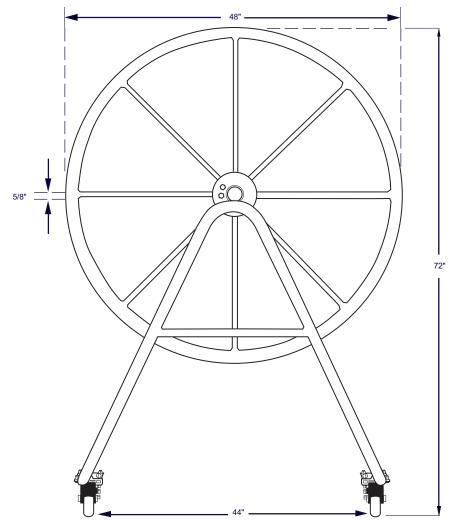
The **"Ultimate"** Storage Reel is large enough to hold a full set of lanes and has unrivalled capacity. The 6'7" long center spool has a diameter of six inches, designed to eliminate the possibility of damage to the discs.
