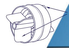
Three fins on both sides of the disc extend fully to engage with adjacent fins, thereby creating a solid wave-retention barrier. No water gets through.
