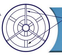
Internal ribs and walls are designed to optimize the impact-reducing capabilities of the disc, while keeping weight to the requisite level.
